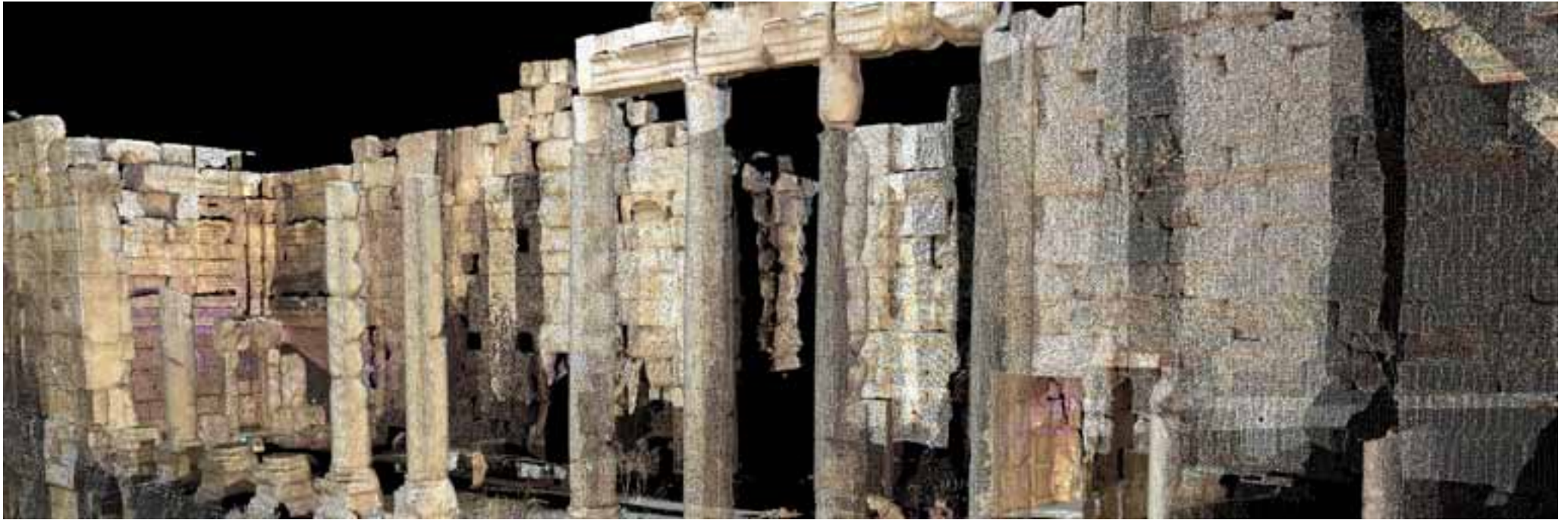
Figure 2: 3D point cloud of the Semi-Circular forecourt and propylaea, by A. Seif, G. Ghattas, Bureau Stéphan and B. Van Genechten.
