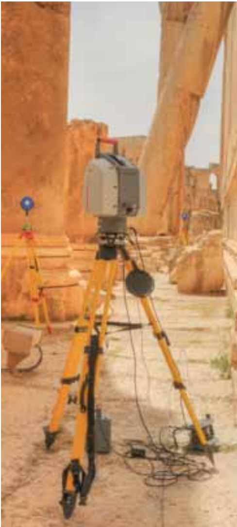
Figure 1: recording in Temple of Bacchus, using the laser scanner in Baalbek, author.
